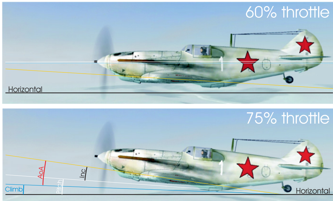
Figure 4.1: In the first picture, Oleg is flying his LaGG-3 in level flight (see section 5.6) at about 310kph. In the second, he has smoothly added throttle and begun to climb. It is clear that the angles of pitch and climb have increased, although the angle of attack has not. The airspeed has not appreciably changed.
